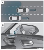
Fig. 163 Schematic representation: A Situation of an overtaking in the centre lane and then moving into the right-hand lane. B Indication of the lane departure warning in the control lamp on the right side.
