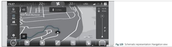
A global satellite system determines the current position of the vehicle and the sensors mounted on the vehicle analyse the routes taken. All measured values and possible traffic events are compared with the available maps to allow optimal navigation to the destination.
