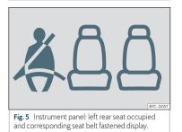
Depending on the model version, when the ignition is switched on, the seat belt status display>>> **Fig. 5** on the instrument panel informs the driver whether the passengers in the rear seats have fastened their seat belts.
