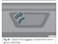
The rear lid can be unlocked from inside in the event of an emergency (e.g. no battery).
