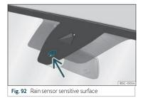
The rain sensor controls the frequency of the windscreen wiper intervals, depending on the amount of rain  $\dots$   $\Delta$ . The sensitivity of the rain sensor can be adjusted manually. Manual wipe $\dots$  page 119.
