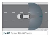
The radar sensors are located on the left and right of the bumper and are not visible from the outside**»** Fig. 143. The sensors monitor both the blind spot and traffic behind the vehicle**»** Fig. 144.
