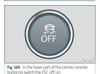
The ESC is switched on automatically when the engine is started, and only works when the engine is running and includes the ABS, EDS and TCS systems.
