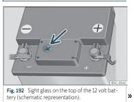
The electrolyte level should be checked regularly in high-mileage vehicles, in hot countries and in older batteries.
