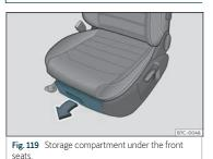
*Opening*: Press the tab on the drawer handle and take the drawer out.
