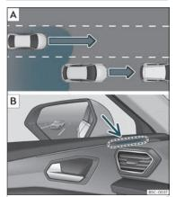
Fig. 162 Schematic representation: A Passing situation with traffic behind the vehicle. B Indication of the lane departure warning in the control lamp on the left side.
