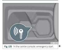
If no valid key is detected inside the vehicle, an emergency start-up will be required. The relevant message will appear in the dash panel display. This may happen when, for example, the vehicle key battery is very low:
