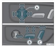
Fig. 96 Driver's seat: electric seat settings.
