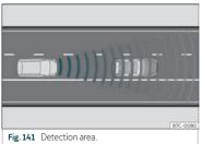
A radar sensor may be fitted to the front bumper of the vehicle>>> Fig. 140. The front radar detects any objects in its detection zone >>> Fig. 141 and provides support for the following functions:
