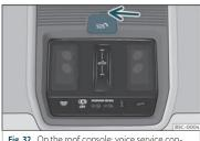
Fig. 32 On the roof console: voice service controls
