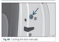
If the central locking system should fail to work at any time, doors with no lock cylinder will have to be locked separately.
