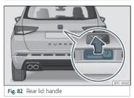
The rear lid opening system operates electrically. It is activated by exerting slight pressure on the handle**» Fig. 82**. To lock or unlock the rear lid, press the  $\rightleftharpoons$  or  $\stackrel{\frown}{\rightrightarrows}$  buttons of the vehicle key.
