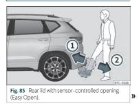
If there is a valid vehicle key in the proximity of the rear lid, it is possible to unlock and open or close it moving one foot in the area of the sensors located under the rear bumper.
