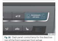
Deactivate the front passenger front airbag only if you have to use a rear-facing child seat in the front passenger seat. CUPRA recommends fitting the child seat in the rear seat to avoid having to deactivate the front passenger airbag.
