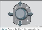
Fig. 99 Detail of the driver's door: control for the exterior mirror.
