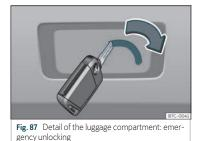
The rear lid can be unlocked from inside in the event of an emergency (e.g. no battery).
