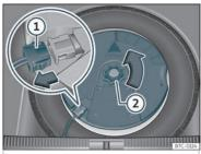
Fig. 214 In the luggage compartment: remove the subwoofer.
