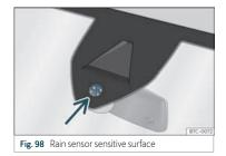
The rain sensor controls the frequency of the windscreen wiper intervals, depending on the amount of rain >>>  $\Delta$ . The sensitivity of the rain sensor can be adjusted manually. Manual wipe>>> page 120.
